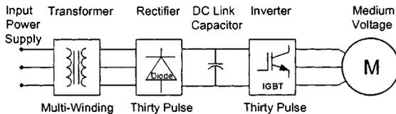
Fig. 4. Medium-voltage multilevel voltage-source inverter (VSI-PWM) drive.
