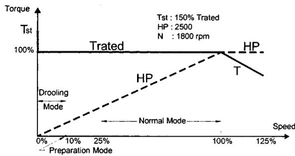
Fig. 1. Extruder torque/speed characteristic.
