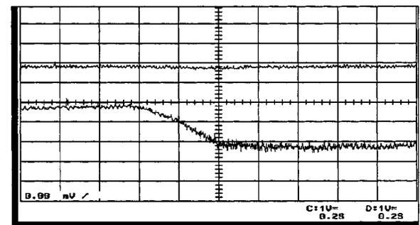
Fig. 7. ASD test at 60 Hz with 100% torque step load. Trace C = torque scaled 5 Vdc = 30 000 in/lb. Trace D = speed scaled 6 Vdc = 60 Hz. Trace C common at center. Trace D common at bottom.
