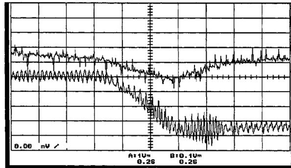
Fig. 5. ASD test at 5 Hz with 100% torque step load. Trace A = torque scaled 5 Vdc = 30 000 in/lb. Trace B = speed scaled 6 Vdc = 60 Hz. Trace A common at center. Trace B common at bottom.
