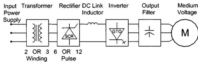
Fig. 2. Medium-voltage CSI with PWM and motor filter capacitors (CSI-PWM).
