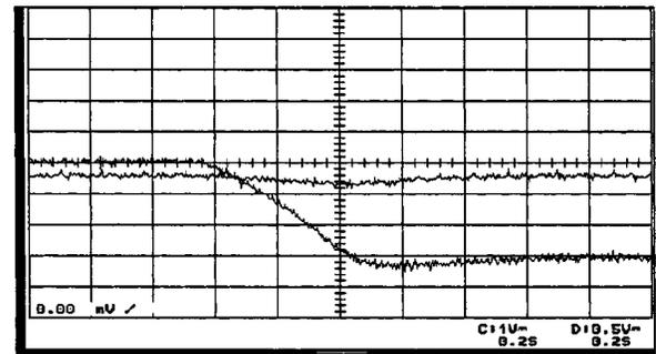
Fig. 6. ASD test at 18 Hz with 100% torque step load. Trace C = torque scaled 5 Vdc = 30 000 in/lb. Trace D = speed scaled 6 Vdc = 60 Hz. Trace C common at center. Trace D common at bottom.
