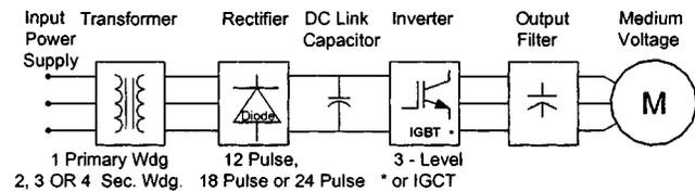
Fig. 3. Medium-voltage three-level voltage-source inverter (VSI-PWM) drive.
