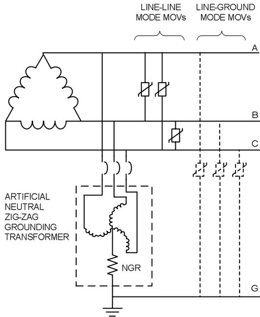
Fig. 3 High Resistance Grounding of a Delta System
