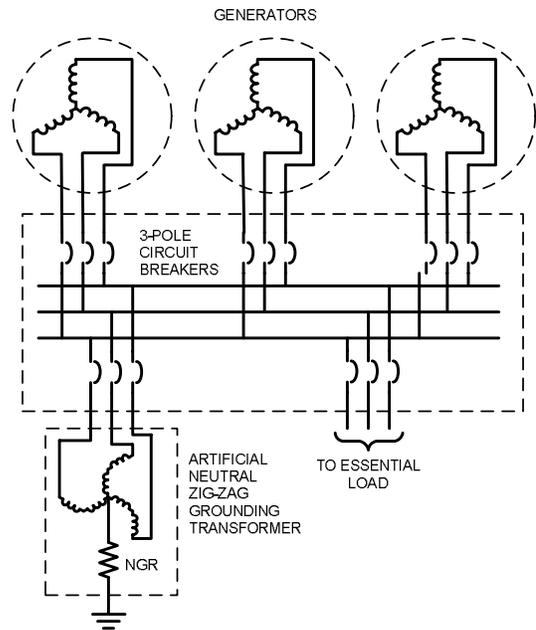
Fig. 7 High Resistance Grounding Scheme of Parallel Generators
