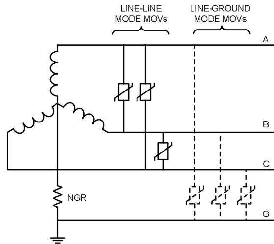
Fig. 2 TVSS for High Resistance Grounded System
