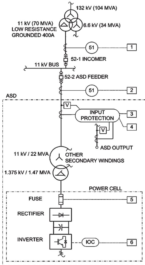
Fig. 5. Protection-coordination single-line diagram.
