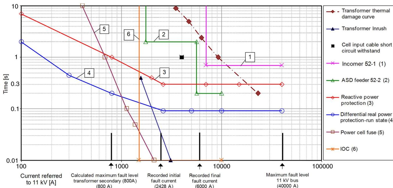
Fig. 6. Protection coordination curves for ASD—all currents shown are referred to 11 kV.
