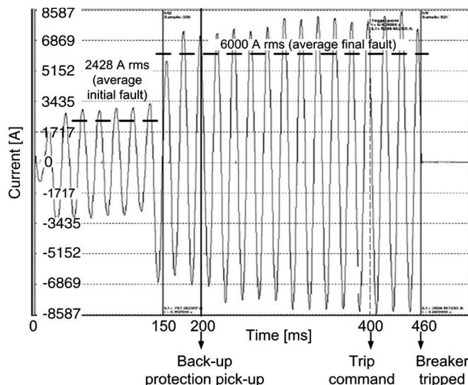
Fig. 3. ASD Feeder (52-2) fault recording at 11-kV side.
