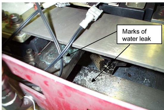
Fig. 4. Power cell A2 showing water marks.
