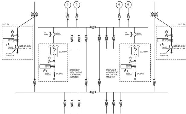
Fig. 3 Two generator busses
