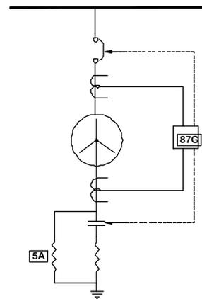
Fig. 7 Hybrid grounding system
