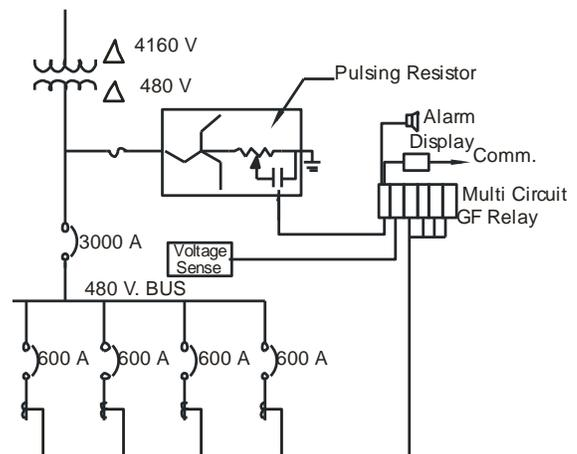
Fig. 1 Typical Delta/Delta installation
