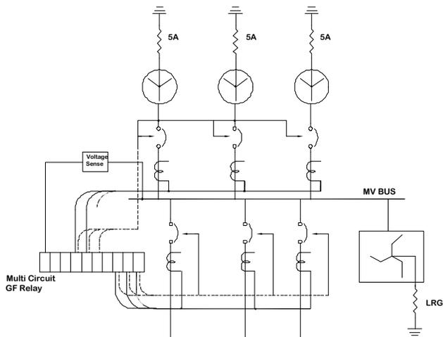
Fig. 6 Extended medium voltage hybrid system
